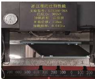
Tensile Force 452 kN/Shear Strain 200% Test Photo
