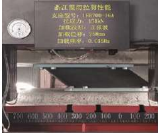
Tensile Force 302 kN/Shear Strain 200% Test Photo
