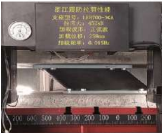
Tensile Force 452 kN/Shear Strain 200% Test Photo
