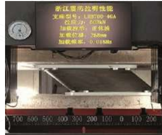
Tensile Force 754 kN/Shear Strain 200% Test Photo
