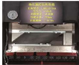
Tensile Force 905 kN/Shear Strain 200% Test Photo
